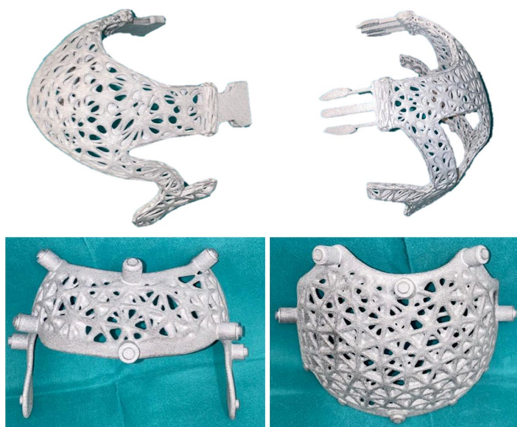
Fig. 9 3D-printed final helmet concept consisting of PA12
