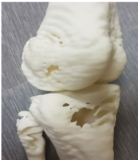
Fig. 8 Image of the 3D-printed prototype illustrating ripple-like effects and hollow areas
