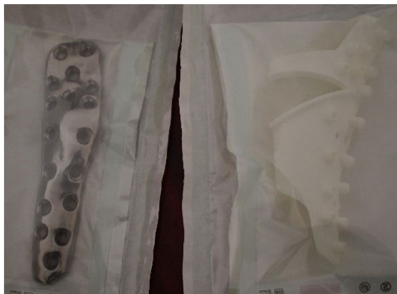
Fig. 6 Implant (Grade23 Titanium-6-Al-4-V) and drill guide received from CUT
