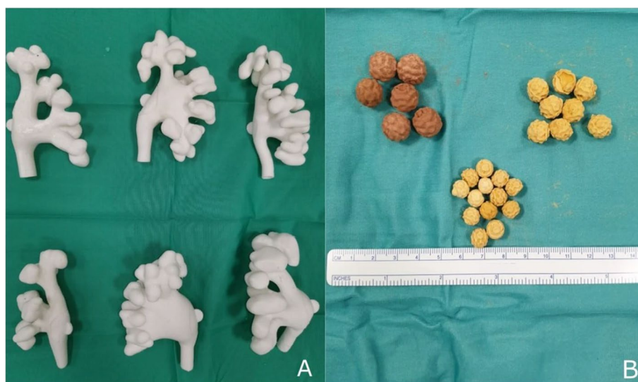
Fig. 3 (A) Three-dimensional printed training models of different pelvic/cecal systems and (B) training stones developed by Orecchia et al. [12]
