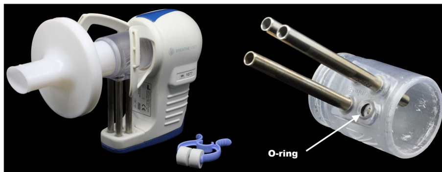
Fig. 4 Left: Assembled breath sampling device comprising the ReCIVA breath sampler (right), a 3D-printed mouthpiece adapter (an adapter made from BioMed Clear resin is depicted; centre), a disposable pulmonary function filter (left), and thermal desorption tubes to sample breath (bottom-centre). The nose clip depicted is used as an adjunct during breath sampling to ensure mouth breathing. Right: Close-up of the underside of the adapter with three inserted thermal desorption tubes and one open tube orifice fitted with an O-ring
