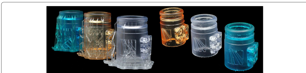
Fig. 3 Final adapter models pictured with (left) and without (right) support structures, printed from Tough v5 (blue), Surgical Guide (orange) and BioMed Clear (translucent) resins
