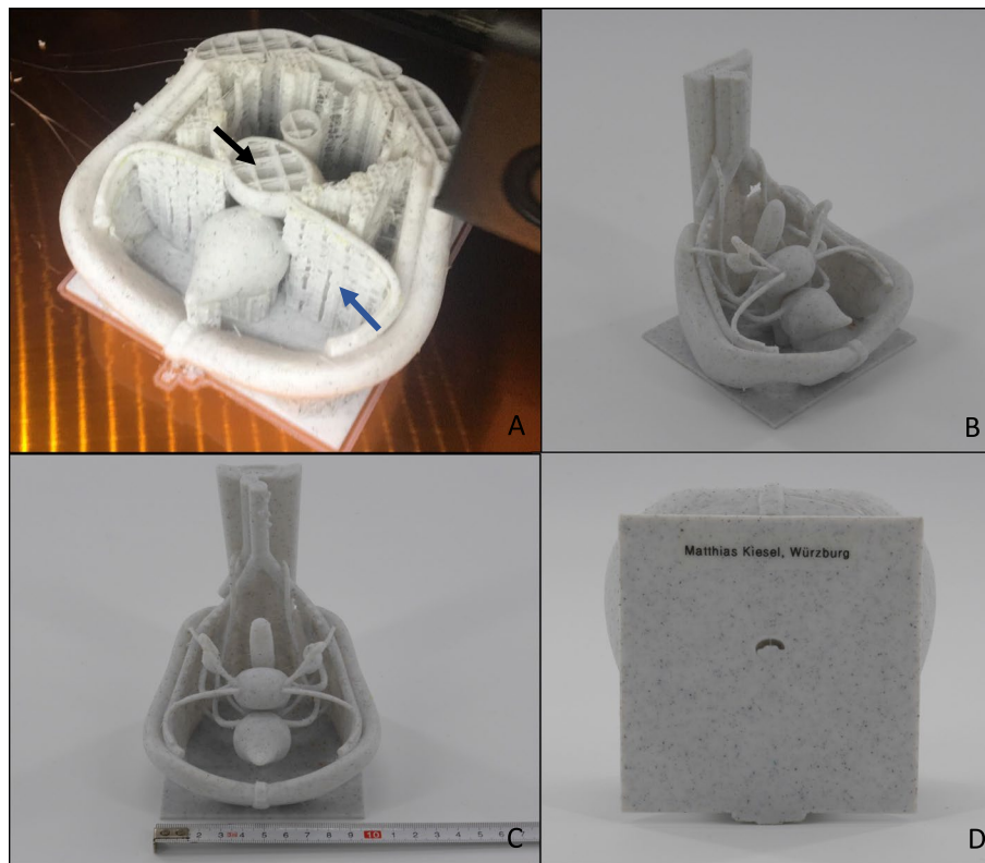
Fig. 6 A-D 3D printed model of the female pelvis, printed in one piece. A Process of 3D printing. 3D printer: Craftbot 3 , company: CRAFTUNIQUE, Budapest, Hungary, filament: PLA, color: Marble, filament-diameter: 1,75 mm from the company Geeetech, Shenzhen, China. Black arrow: relatively low density of infill material can be seen, as the inside of the model is not printed of massive PLA. This accelerates the printing-process and reduces the amount of filament needed at the cost of stability. Blue arrow: support material, which has to be removed manually after the print. B Finished model directly after being removed from the 3D printer. Support material still remaining. C Measure showing the size of the model (10 cm width). D Vulva and openings for urethra, vagina and anus have not yet been printed
