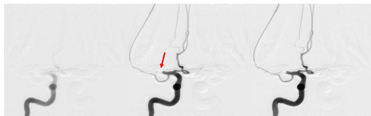
Fig. 6 Angiograms were taken post-stent retriever thrombectomy for each of the cases. A successful case and an unsuccessful case are displayed above. The successful case shows contrast flowing through the neurovascular phantom resulting in no occlusion. While the unsuccessful case shows the contrast flow being halted where the blood clot is still blocking the vessel resulting in full occlusion (red arrow)
